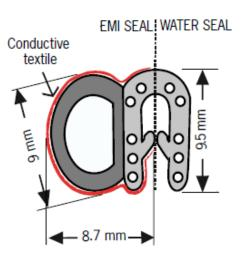
Part No: K\_6562 Clamping Range: 1 to 3 mm Material: EPDM 60 ±5 shore A Part No: K\_6595 Clamping Range: 0.5 to 2 mm Material: EPDM 60 ±5 shore A
