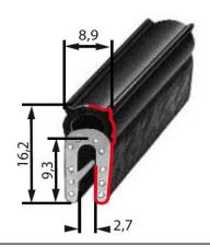
Part No: K\_6566 Clamping Range: 0.5 to 2 mm Material: EPDM 60 ±5 shore A
